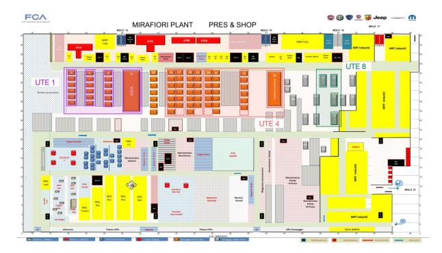
Figure 34: CRF Plant Layout
